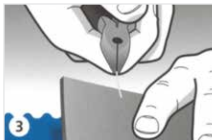
Gently pull the pin out using pliers.
