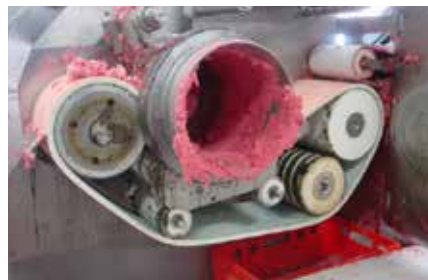
Separating application in a meat production line.
