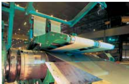
Coil wrapping application in a sheet metal production line.
