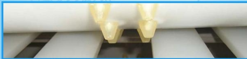
Typical Cog-Veyor bed showing drive lug arrangement and UHMW support strips
