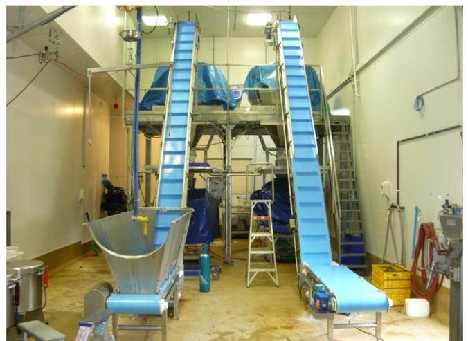
Both conveyors are now running Cog-Veyor belts and the client is very pleased with the outcome. The positive drive of the belts ensure smooth quiet operation, and our unique self tracking lugs, ensure the belt runs true, with no maintenance or downtime.
