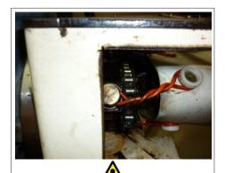
Inferior rings can stretch, break and fall off into the frame or worse... .....into your product
