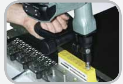
Electric Powered Rivet Driver Installation
