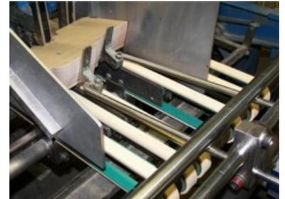
**Ultrafeed 500** feeder belts in operation
